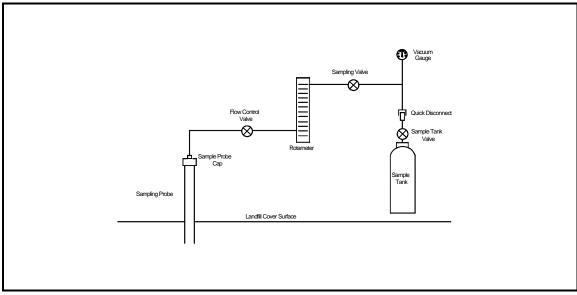
Figure 25C-2. Schematic of Sampling Train.
